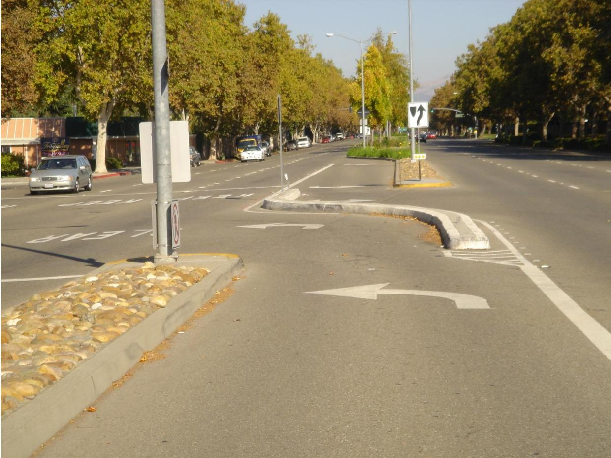
Commentary: A 4-way Intersection of a major urban arterial was created when a driveway was located directly opposite a collector street. A barrier eliminates crossings and left-turns onto the urban arterial.
