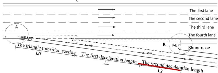
Schematic deceleration of the lane length calculation
