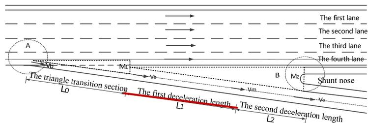
Schematic deceleration of the lane length calculation
